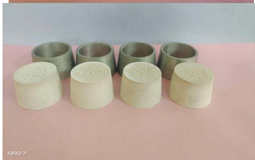
Fig. S-2. Compressive and setting time blocks without cracking.
