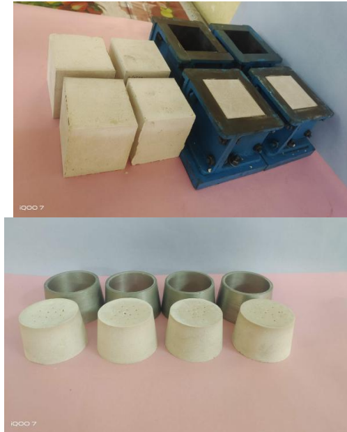
Fig. S-2. Compressive and setting time blocks without cracking.
