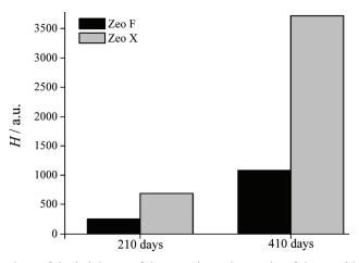
Fig. S-1. Comparison of the heights *H* of the most intensive peaks of the two identified zeolite phases, zeolite X and zeolite F, after 210 and 410 days of alkali treatment.
