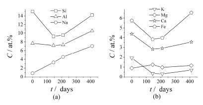
Fig. S-2. Content *C* of Na, Al and Si (a) and K, Ca, Mg and Fe (b) in the reaction products as a function of the time *t* of alkali treatment of the finer S fraction.
