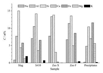
Fig. S-3. Elemental composition of the initial slag, the reaction products (sample S410), and of the crystallites of two zeolite phases X and F (Zeo X and Zeo F) formed after 410 days of alkali activation. For comparison, the respective data for the amorphous precipitates obtained after the same treatment time of the coarser fraction L are also presented.
