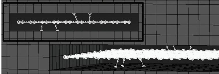
Fig. S-9. Nanocomposite reinforced by a monolayer GS and bidirectional covalent bonds as interlayer interactions.
