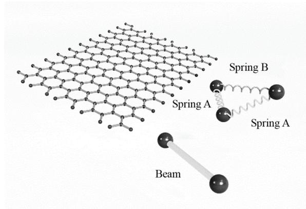
Fig. S-1. Definition of the mechanical elements.
