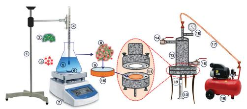
(1) Stand, (2) PVA (3) Formaldehyde, (4) Thermometer, (5) Distilled water, (6) Magnetic Bar, (7) Magnetic Stirrer, (8) Formaldehyde crosslinked PVA, (9) Coated Crosslinked PVA on support, (10) Flyash support, (11) Sandwich structure of Composite membrane, (12) Dead-end membrane filtration setup, (13) Measuring cylinder, (14) Feed valve, (15) Retentate outlet valve, (16) Pressure gauge, (17) Gas tube, (18) Air compressor, (19) Permeate outlet
