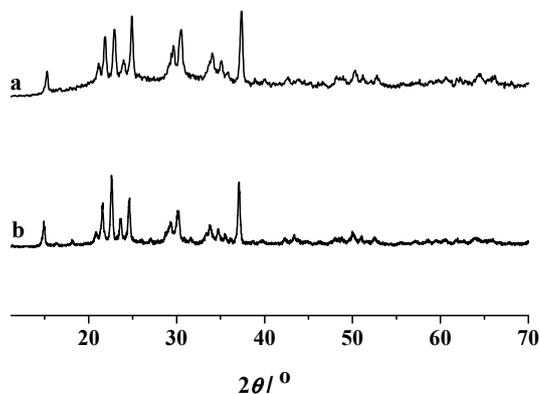
Fig. S-1. XRD patterns of: a) the fresh WG-2.0 and b) the five times reused WG-2.0.
