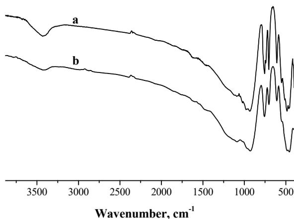
Fig. S2. FTIR of: a) the fresh WG-2.0 and b) the five times reused WG-2.0.
