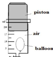
In this figure, a moderately swollen child's balloon has been placed within a free-piston injector that contains a little air and a closed end. Accordingly, which of the following statements are true?
