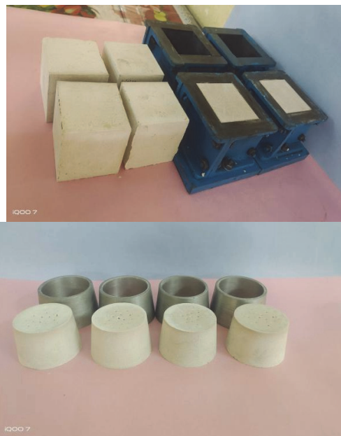
Fig. S-2. Compressive and setting time blocks without cracking.
